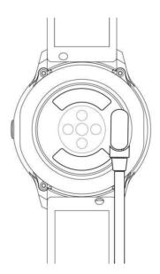
\*Be aware that the two contacts of the USB cable are not allowed to contact the conductor at the same time, or it will cause the circuit to burn.
